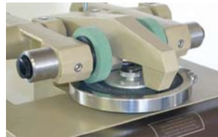
The Taber Rotary Platform Abraser
